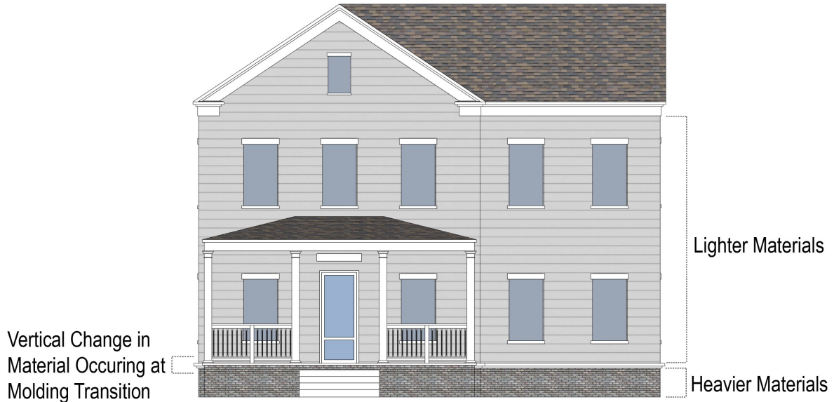
Figure 27-24-31: Residential building material and details
