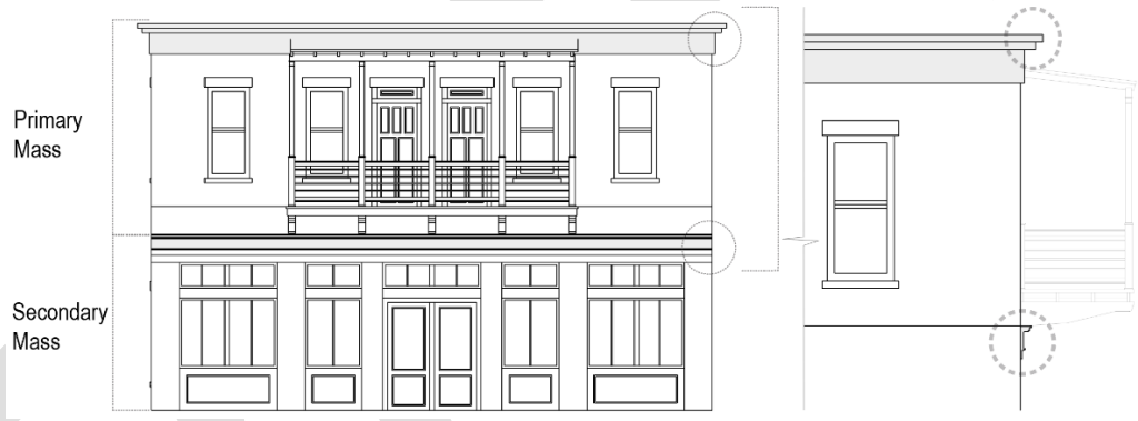
Figure 27-246-8: Building with a primary and secondary cornice.
