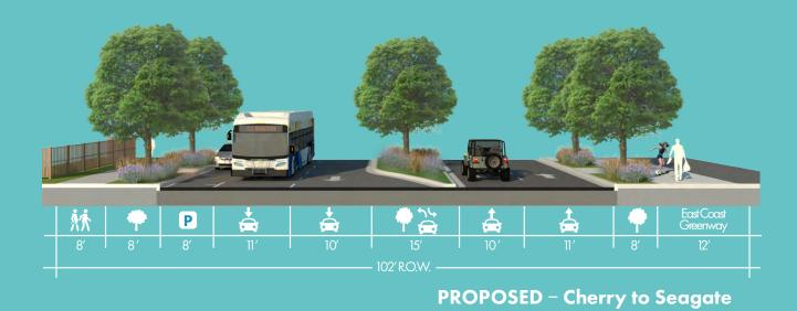
Figure 4.14: 3rd Street/A1A Proposed Street Sections
