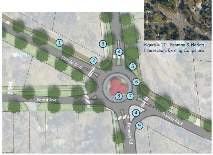
Figure 4.21: Penman & Florida Intersection: Proposed Roundabout Plan
