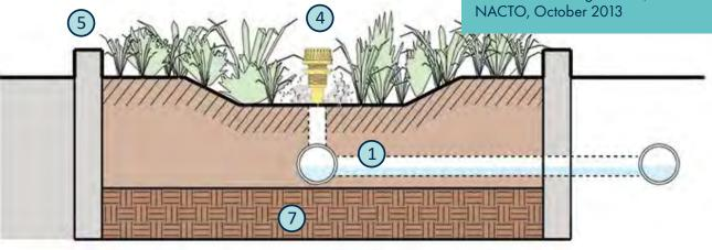
Figure 4.90: Section of a bioswale. Image courtesy of National Association of City Transportation Officials (NACTO)
