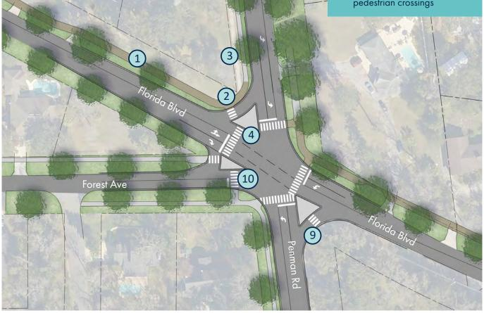
Figure 4.23: Penman & Florida Intersection: Proposed Signalized Intersection Plan
