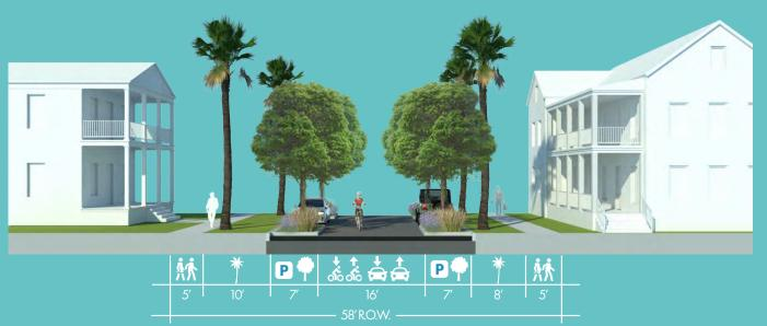
Proposed – Option B: The pavement width and curbs remain the same, however the street becomes one-way with a cycle track on the eastern side and on-street parking with pervious pavers on the left side. The on-street parking will have bulb outs with bioswales and shade trees and native landscaping to filter and absorb stormwater runoff.
