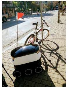
Figure 4.54: Delivery Robot
