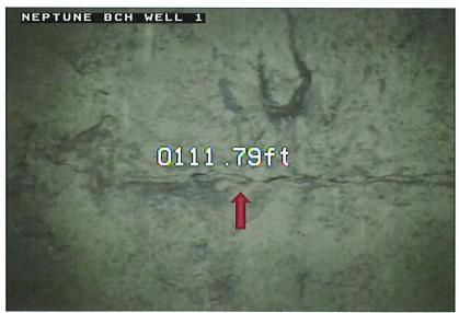
Photograph 2 - Typical Casing Joint at 111 feet
