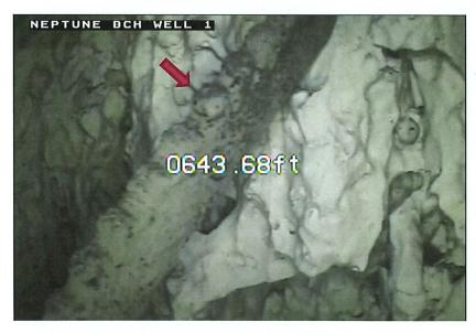
Photograph 5 - Metal Strap/Rod Observed in Well
