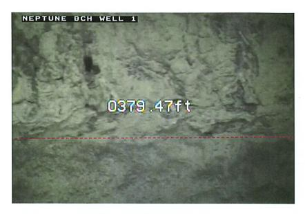
Photograph 6 -Bottom of Casing Side View
