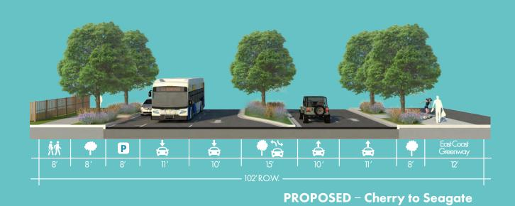
Figure 4.14: 3rd Street/A1A Proposed Street Sections
