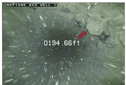
Photograph 3 - Casing Incrustations (Looking Down in to Well)
