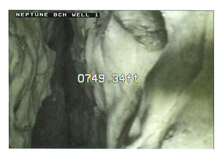
Photograph 7 - Water-Bearing Fractures and Voids in Open Hole
