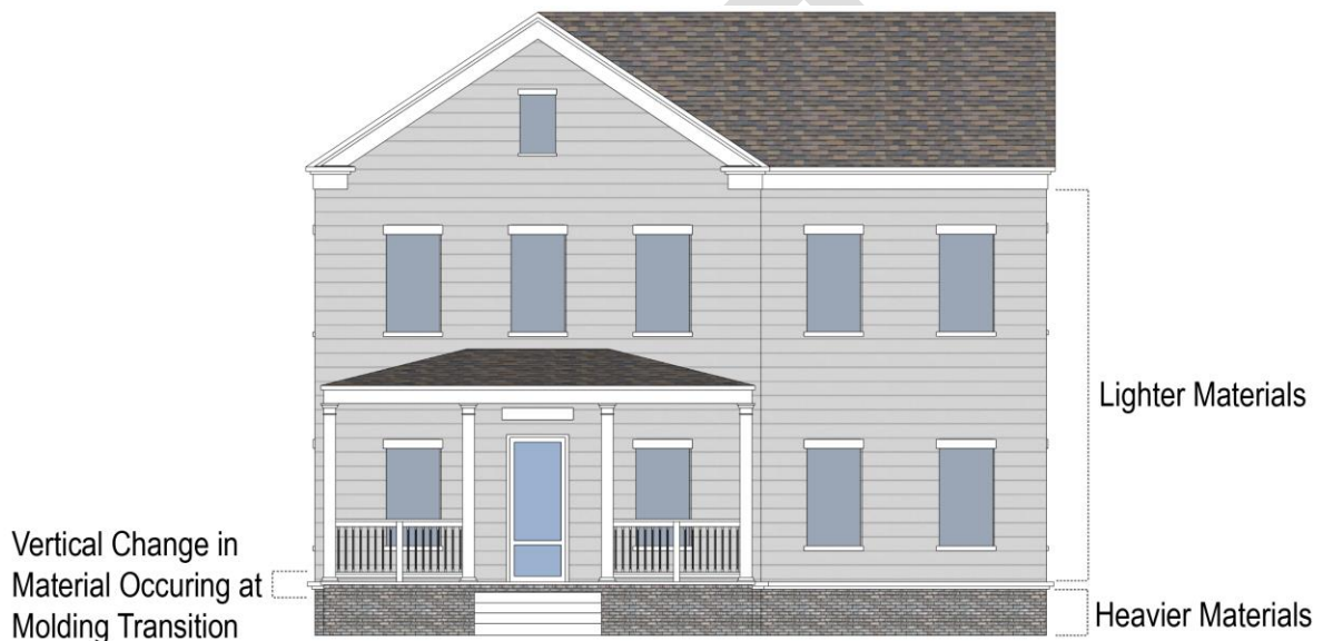
Figure 27-243-1: Residential building material and details
