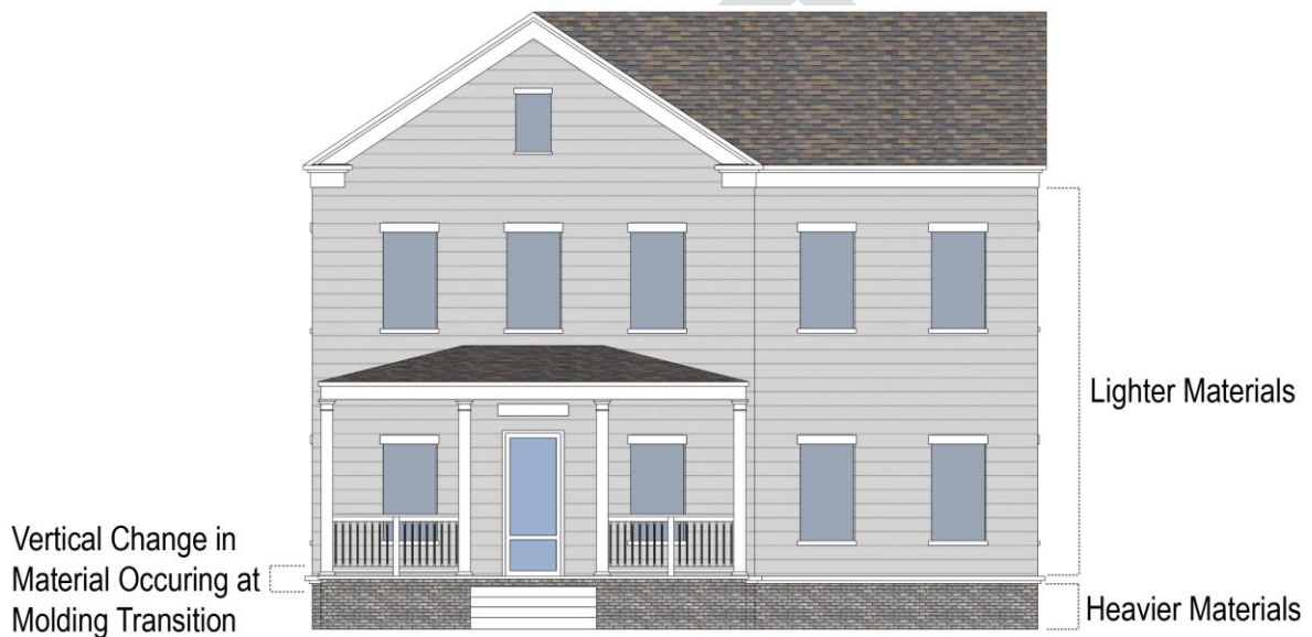
Figure 27-243-1: Residential building material and details
