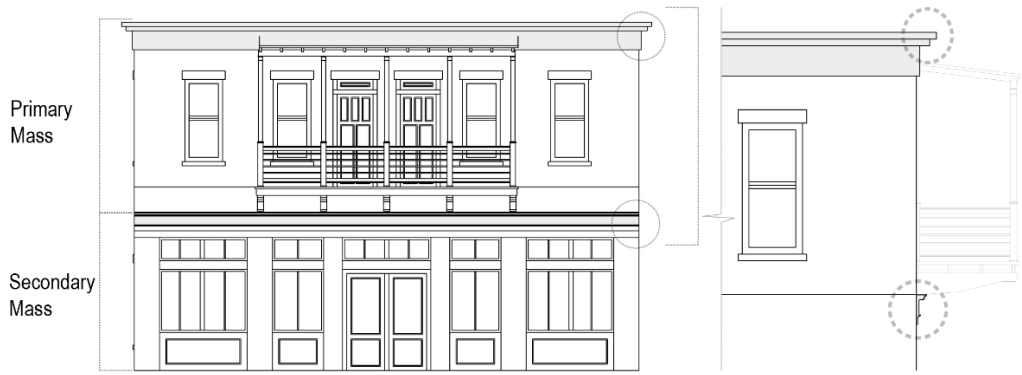
Figure 27-246-8: Building with a primary and secondary cornice.
