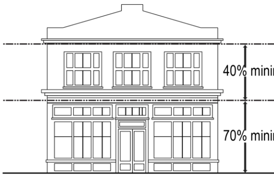
Figure 27-246-3: Façade transparency requirement for buildings with
