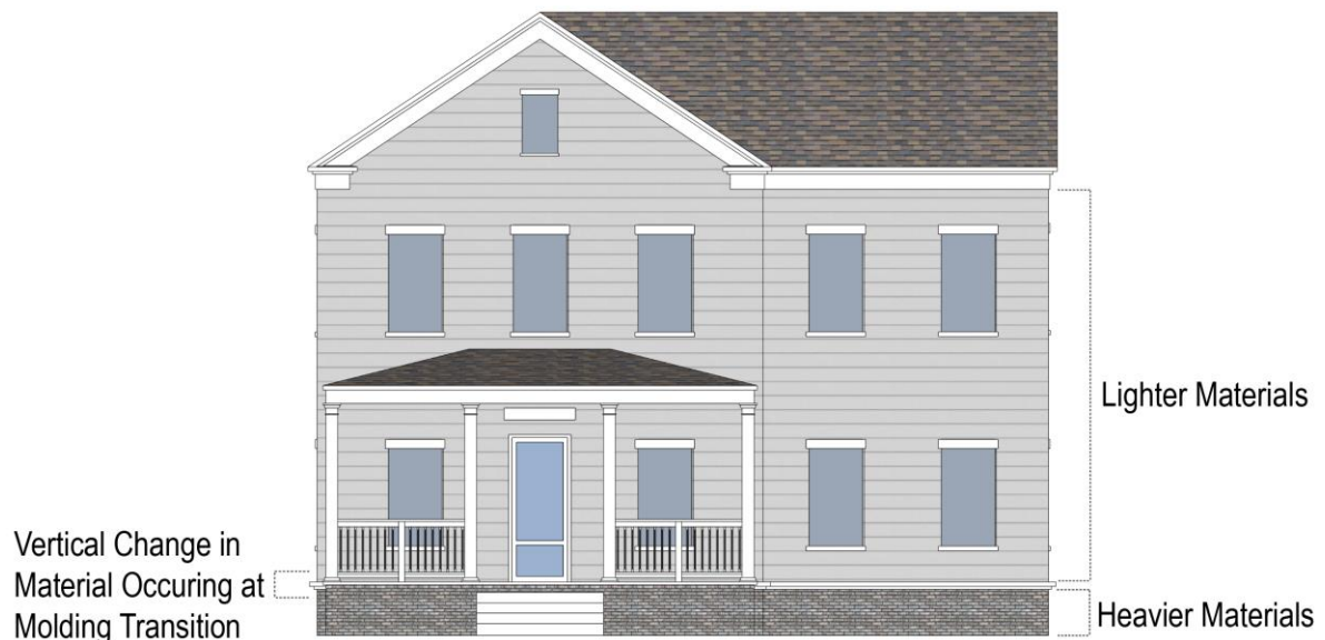
Figure 27-243-1: Residential building material and details
