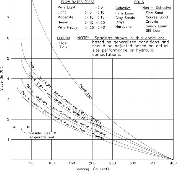
CHART RECOMMENDED SPACING FOR TYPE I AND TYPE II HAY BALE BARRIERS, AND TYPE III AND TYPE IV SILT FENCES AND PAVED DITCH HAY BALE BARRIERS
