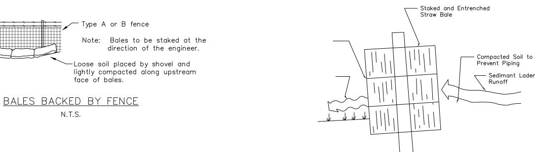
CROSS-SECTION OF A PROPERLY INSTALLED STRAW BALE
