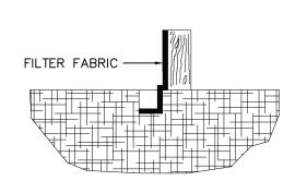
CONSTRUCTION DETAILS FOR SILT FENCES (D-909) N.T.S.
