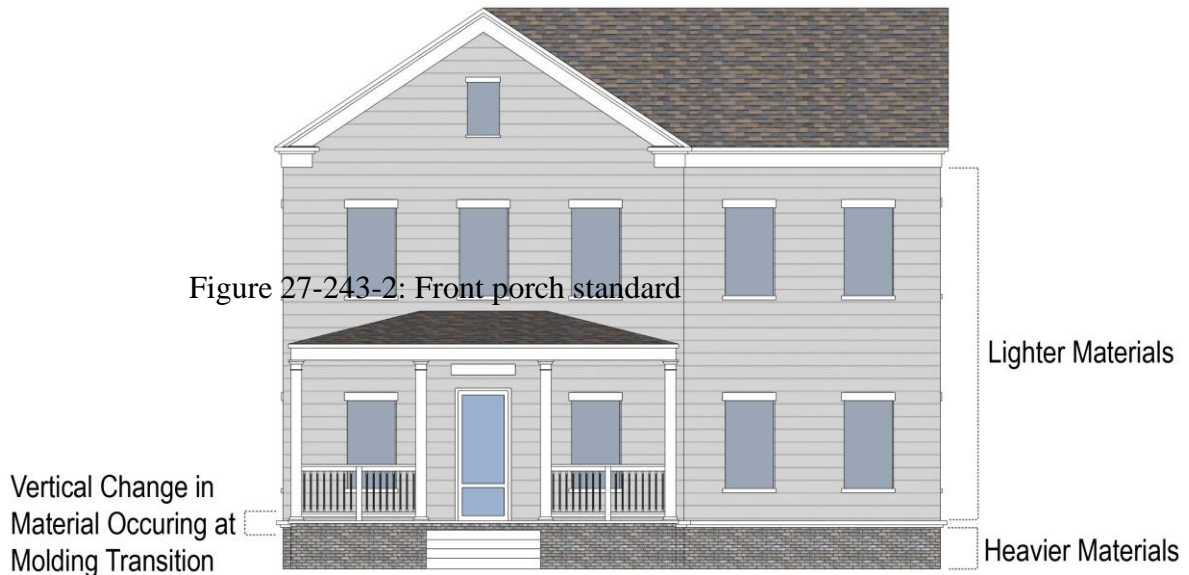
Figure 27-243-1: Residential building material and details
