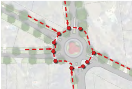
Figure 4.24: Roundabout: Pedestrian Route and Stops
