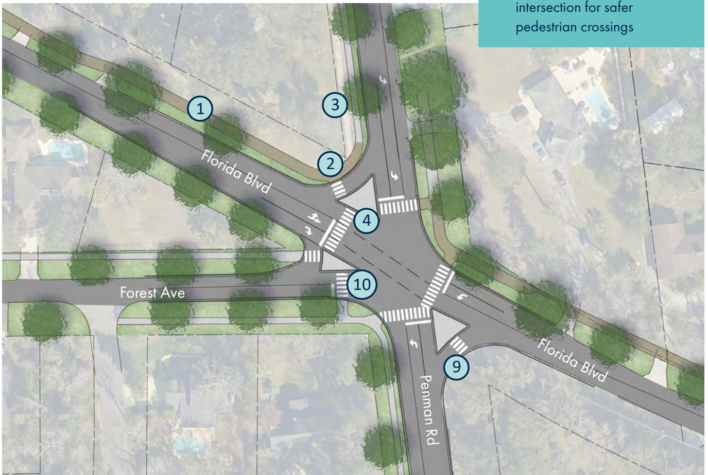
Figure 4.23: Penman & Florida Intersection: Proposed Signalized Intersection Plan
