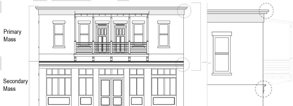
Figure 27-246-8: Building with a primary and secondary cornice.
